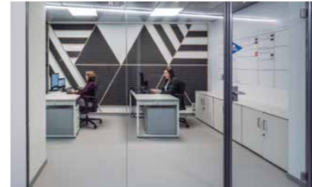
Dark areas can be visible when the dimming level is lower than 40%
